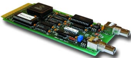
FIG 3. Single Time Code Encoder Module
